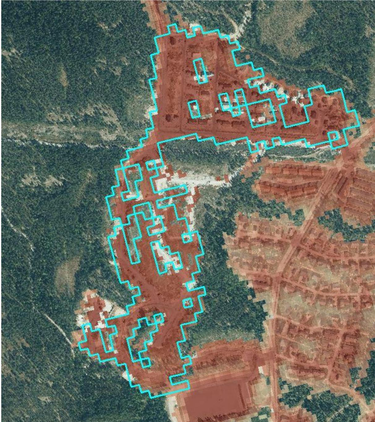
Figure 14. Commission errors in the bottom half of the construction area: HRL IMD18 data shows impervious (shades of red), but no structures are yet present. The turquoise polygon is the contradicting area derived from the GIS comparison of in-situ data and the HRL IMD18. SAMPLE\_ID 67, scale 1:5000, coordinates (ETRS\_1989\_LAEA) E:5033247, N:4332586, orthophoto reference year 2018.
