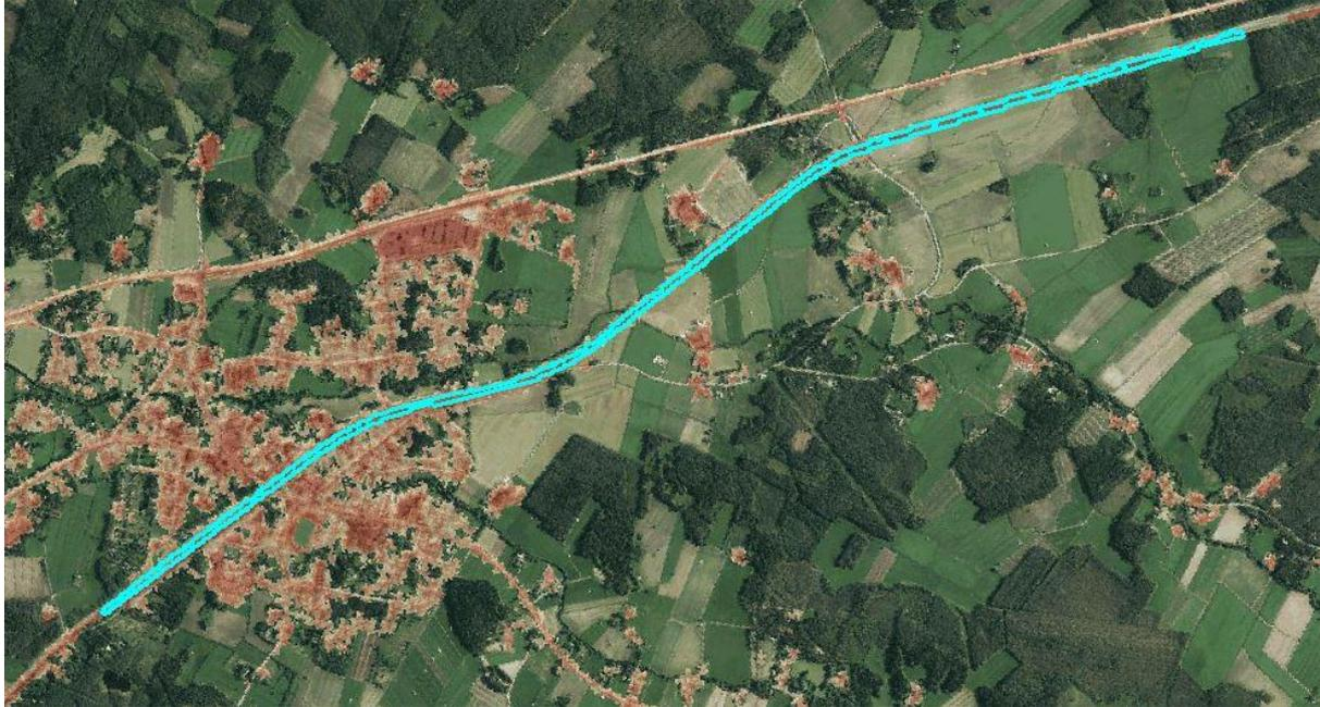
Figure 23. Parts of the railway tracks located outside the urban area are misclassified as impervious. The turquoise polygon is the contradicting area derived from the GIS comparison of in-situ data and the HRL IMD18. HRL IMD18 data is presented with shades of red. SAMPLE\_ID 201, scale 1:20000, coordinates (ETRS\_1989\_LAEA) E:4983158, N:4592834, orthophoto reference year 2018.
