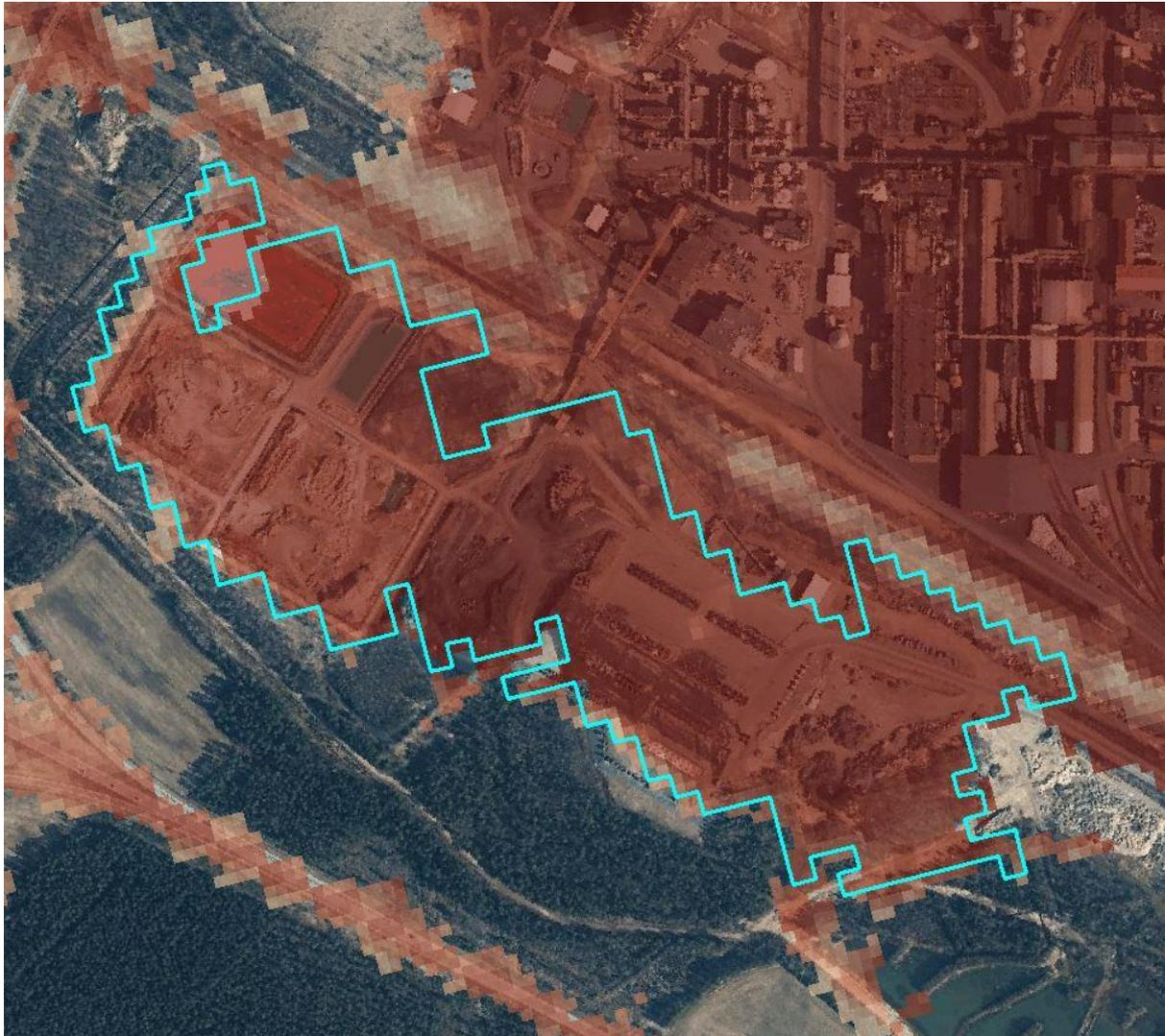
Figure 17. A dump site, that is mostly misclassified as impervious. The turquoise polygon is the contradicting area derived from the GIS comparison of in-situ data and the HRL IMD18. HRL IMD18 data is presented with shades of red. SAMPLE\_ID 111, scale 1:4000, coordinates (ETRS\_1989\_LAEA) E:4968158, N:4301985, orthophoto reference year 2019.
