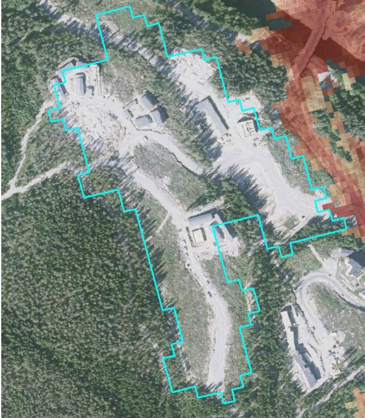
Figure 12. Buildings omitted in a construction site. The turquoise polygon is the contradicting area derived from the GIS comparison of in-situ data and the HRL IMD18. HRL IMD18 data is presented with shades of red. SAMPLE\_ID 59, scale 1:3500, coordinates (ETRS\_1989\_LAEA) E:5215133, N:4529817, orthophoto reference year 2018.
