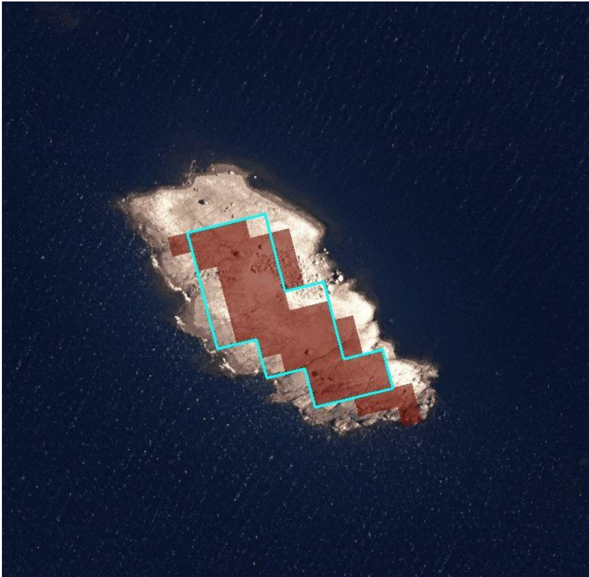
Figure 19. An example of a commission error on a small rocky island. The turquoise polygon is the contradicting area derived from the GIS comparison of in-situ data and the HRL IMD18. HRL IMD18 data is presented with shades of red. SAMPLE\_ID 137, scale 1:1500, coordinates (ETRS\_1989\_LAEA) E:5258617, N:4260533, ortophoto reference year 2017.
